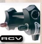
RCV (Open Bath) The CV is the evolution of the super reliable SSVF. The new CV is an easy to use compression adjustment to control the compression rate in one leg teamed up with a separate rebound adjustment in the opposite leg.
