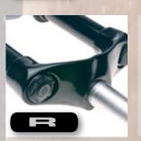
Perfect for beginners or bike enthusiasts, the R valve is the basic rebound adjustment used to control the extension rate. Adjustable from the bottom keeps the
